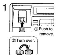
Remove the handset guide from the unit, then turn it over.
